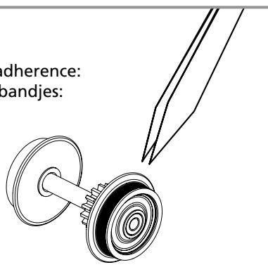
If used frequently, oil the wheelsets with a drop of non-resinous, acid-free sewing machine oil! In order to achieve the best possible running and traction properties, it is advisable to run the locomotive in forward and reverse directions without load. Clean rails are essential for good performance.
